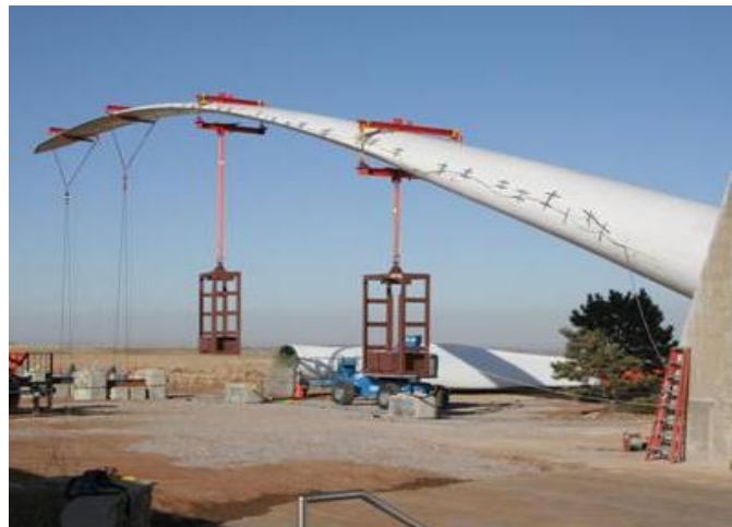
Figure 1.7 Static Testing using ballast weights and winches
